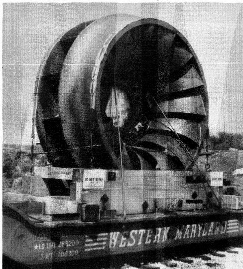
Figure 6: A Francis water-turbine runner.
